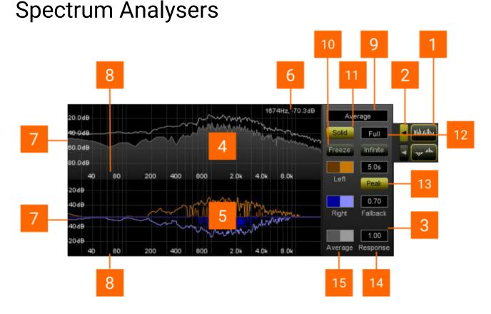
The spectrum analyser views are turned on using the spectrum analyser View Selector Controls [1]. The adjustable parameters are displayed on the Edit Control Panel [3] which is accessed via the adjacent Edit Selector Control [2].
