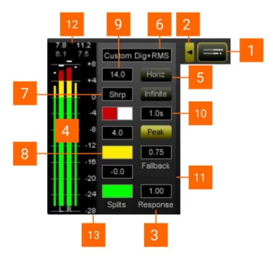
The level meter view is turned on using the level meter View Selector control [1]. The adjustable parameters are displayed on the Edit Control Panel [3] which is accessed via the adjacent Edit Selector control [2].
