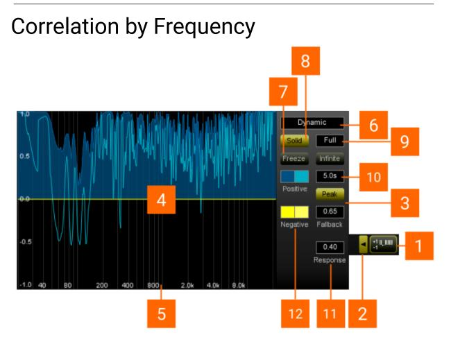
The correlation meter view is turned on using the correlation meter View Selector control [1]. The adjustable parameters are displayed on the Edit Control Panel [3] which is accessed via the adjacent Edit Selector control [2].
