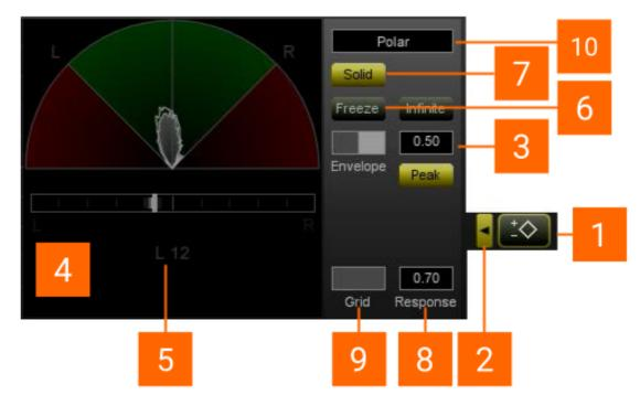
The Vectorscope view is turned on using the Vectorscope View Selector control [1]. The adjustable parameters are displayed on the Edit Control Panel [3] which is accessed via the adjacent Edit Selector controls [2].
