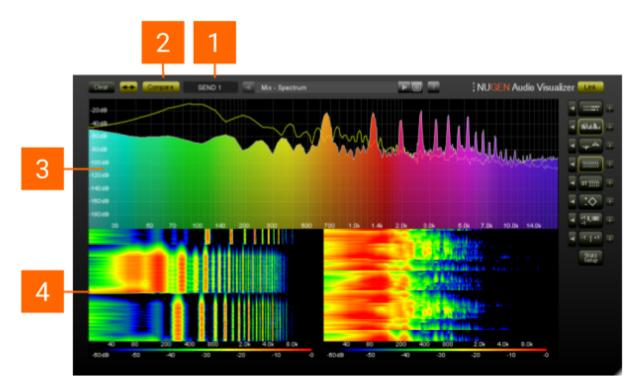
1 Attached 'SEND' plug-in. If more than one SEND is available, click here to choose from a drop-down list. The SEND plug-in is used as a side-chain audio reference to provide the secondary audio source for comparison.
