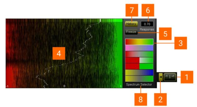
The correlation meter view is turned on using the correlation meter View Selector control [1]. The adjustable parameters are displayed on the Edit Control Panel [3] which is accessed via the adjacent Edit Selector control [2].
