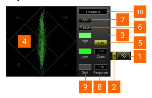
The Vectorscope view is turned on using the Vectorscope View Selector control [1]. The adjustable parameters are displayed on the Edit Control Panel [3] which is accessed via the adjacent Edit Selector control [2].
