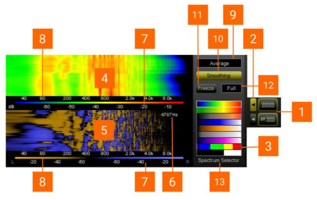
The spectrogram views are turned on using the spectrogram View Selector controls [1]. The adjustable parameters are displayed on the Edit Control Panel [3] which is accessed via the adjacent Edit Selector control [2].
